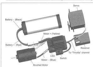
"+" and "-" wires of the ESC are connected to the battery pack.
